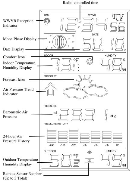
**B.** There are many different modes the indoor weather station can be set to. The LCD shown is the normal operating mode, and your actual data shown will be different based on your local settings and conditions.
